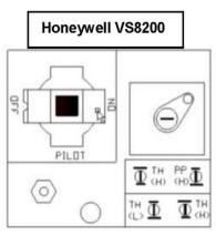
3. While pressing the knob down, use a lit match to ignite the pilot. Continue to press the knob down for about 30 seconds. If the pilot does not stay lit when the
